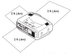
Do not place objects in the areas along the left, back and front sides of the projector For ceiling mount applications, this area should be 5 feet (1.5m).
